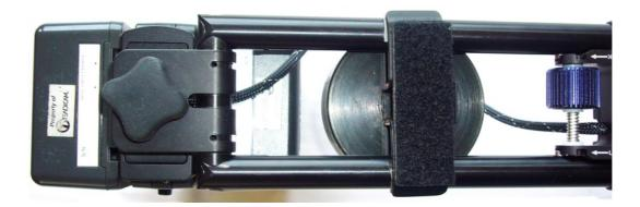
...and you have two useful accessory plates that can remain on the rig secured by quarter-twenty screws when the weights themselves are not required. If velcro is not enough, you can screw up through a quarter inch hole in the top surface of the clamp into any device you want to fix securely.
