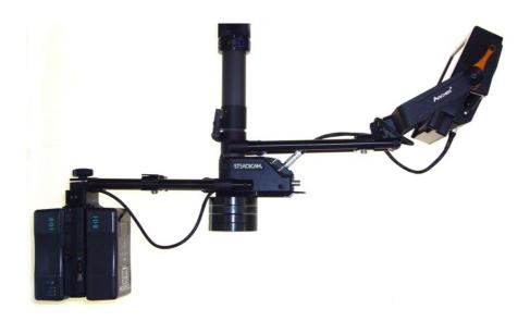
If the camera you are using is too light for your rig, you can add weight above by screwing the weights directly into the camera handle, as shown. (Never add more weight to the handle than the weight of the camera itself.)
