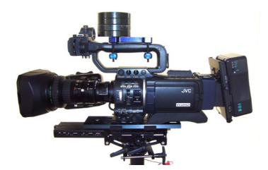
If your camera doesn't have a thread on the handle, use the camera handle Low-Mode Bracket, like this. The farther the weight from the gimbal, the more effective the counterbalance.
